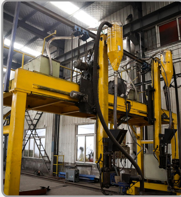
Boxed Submerged Arc Welding
