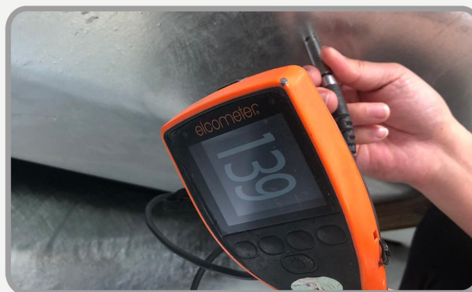
Zinc Thickness Checking
